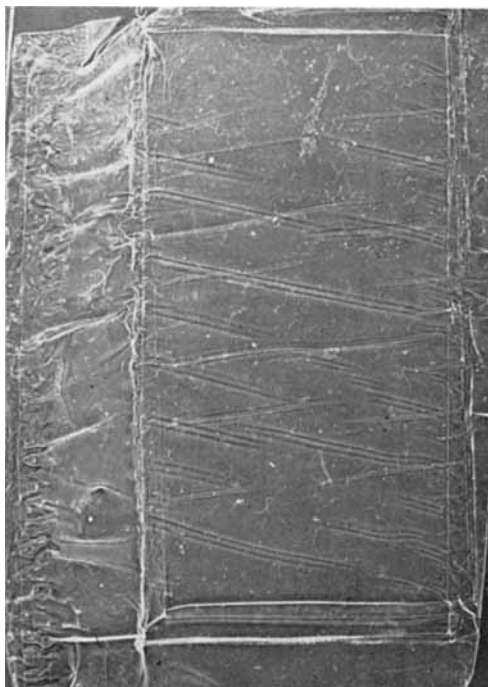
Fig. 1. Kel-F film, 66\ \mu thick, showing the formation of multiple creases in parallel lines under the action of the heat.
